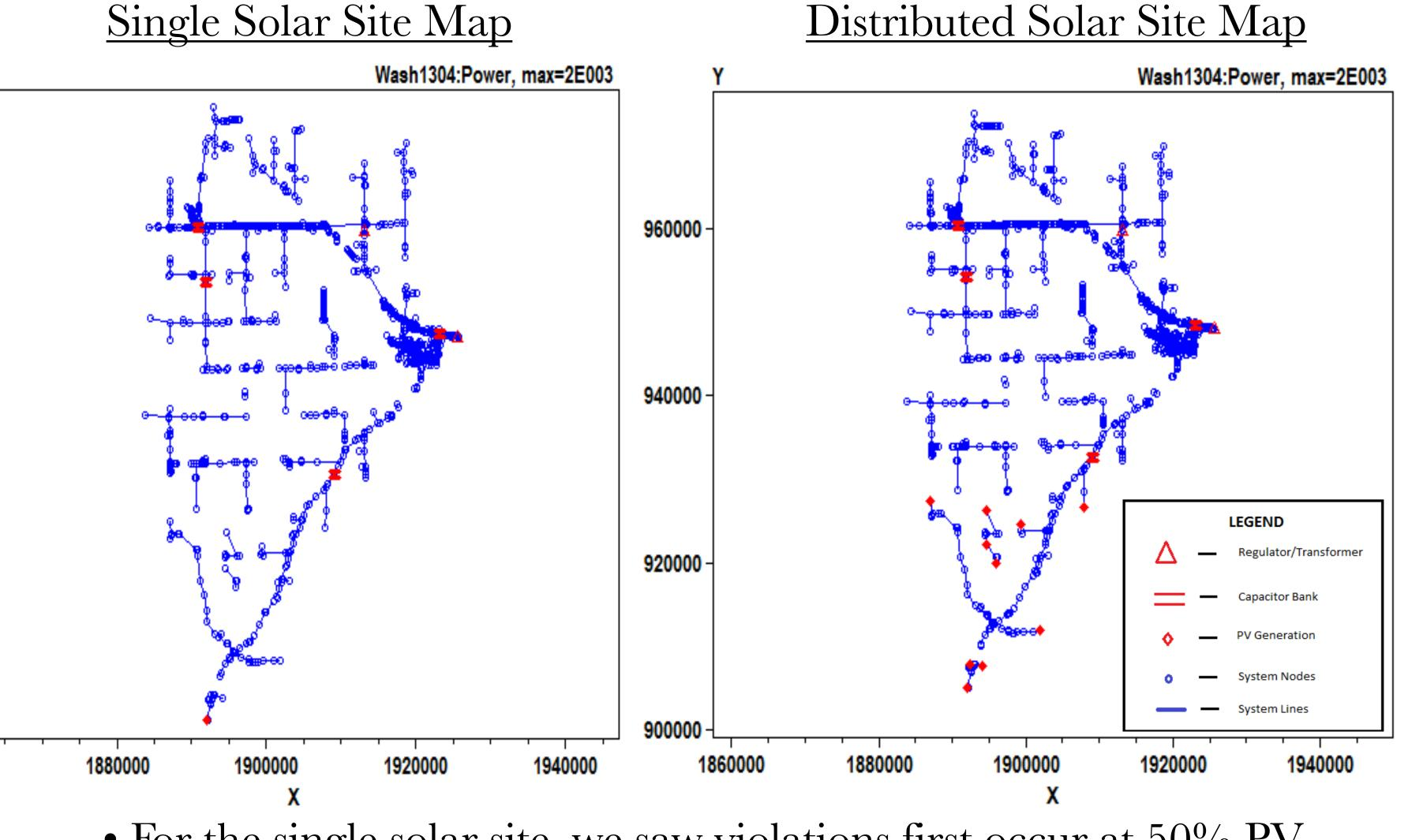
• For the single solar site, we saw violations first occur at 50% PV penetration. For this case, with cloud cover, addition of a smart
